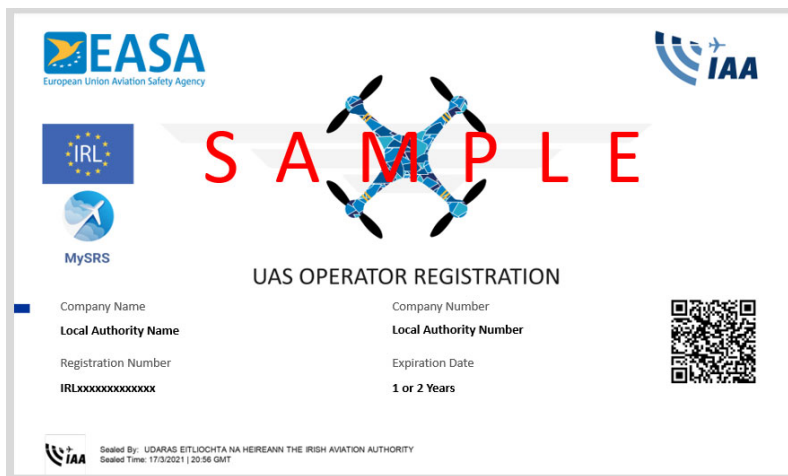
Example of the UAS Operator registration certificate. Note the Registration number. This alphanumeric here should be affixed to the frame of all unmanned aircraft used by a UAS Operator.
